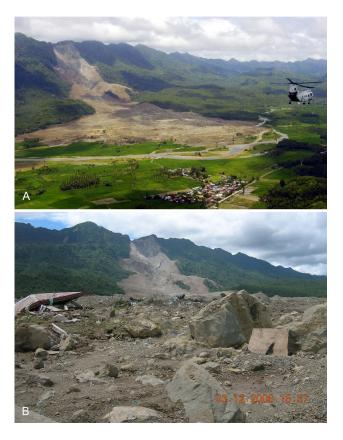
**Fig. 1.** (**A**) Oblique aerial view (to the northwest) of the Guinsaugon landslide taken on 19 February 2006. (U.S. Navy photograph by M. D. Kennedy). The Himbungao River flows from right to left. (**B**) View of debris toward the source area of the rockslide-debris avalanche (Photograph taken 12 March 2006).
