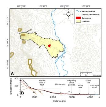
**Fig. 6.** (A) Map of area of Guinsaugon landslide based on SRTM data. Holes are apparent in the digital terrain data along the ridge line (see Appendix for discussion). Outline of the landslide is based on interpretation of ASTER image collected on 1 March 2006 and GPS-controlled field traverses in March 2006. (B) Profile of rockslide-debris avalanche based on SRTM data and field measurements in March 2006. Line of profile is marked in Fig. 6b (S-S').
