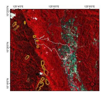
**Fig. 7.** Satellite image of the landslide site (SPOT image, June 2003) with outline of the rockslide-debris avalanche (from Fig. 6a) showing pre-event conditions on the source slope and in the Himbungao river valley.
