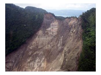
**Fig. 8.** Aerial view of the sliding surface showing horizontal striations consistent with strike-slip fault movement. Note also rock mass characteristics on the right of the source area resulting from movement of Philippine Fault (Photograph courtesy of Mines and Geosciences Bureau, Government of the Philippines).
