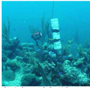
determined by weighing the residue. Light transmission is also used to determine the amount of sediment in the water column. Longer term studies involve the use of sediment traps which are placed on or near the bottom to collect sediment settling out of suspension. These are collected periodically and the sediment is recovered to determine deposition rates.
